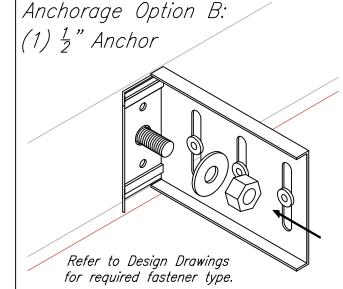
Install screws using a screw gun that does not exceed 2,500 rpm. #12 Screws Screw gun must be equipped with torque limiting clutch to avoid fastener overdrive.
