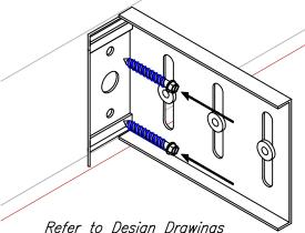
Refer to Design Drawings for required fastener type.
