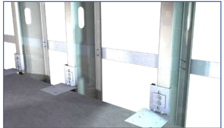
VertiClip SLF used with one flat strap brace on the outer flange of studs to resist torsional effects.
