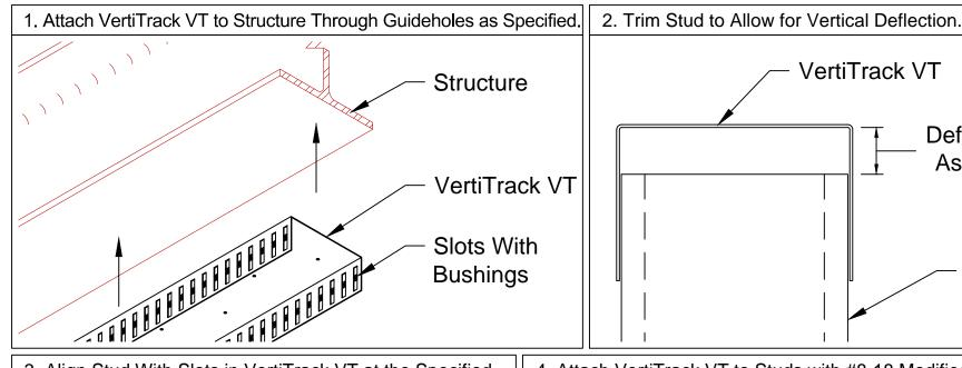
3. Align Stud With Slots in VertiTrack VT at the Specified Stud Spacing.
