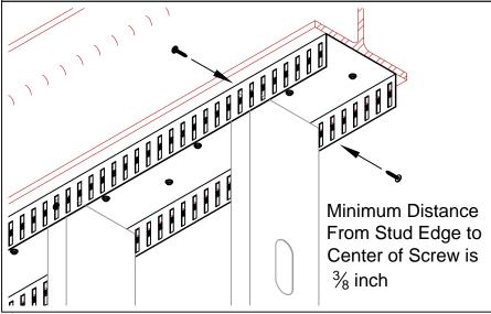
4. Attach VertiTrack VT to Studs with #8-18 Modified Truss Head Screws Through Bushings in Each Flange.
