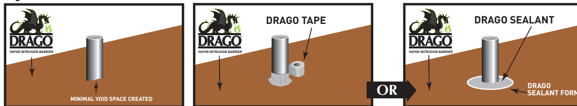
Fig. 4a: PIPE PENETRATION SEALING
