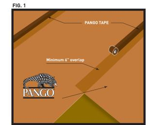
Pango Wrap can be installed over an aggregate, sand, or tamped earth base. It is not necessary to have a cushion layer or sand base, as Pango Wrap is tough enough to withstand rugged construction environments.
