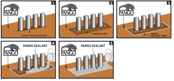
NOTE: For the toughest, hardest-to-reach clusters of multiple pipes or penetrations – Pango Sealant used with Pango Claw and Pango Sealant Form provide an efficient way to achieve a seal.
