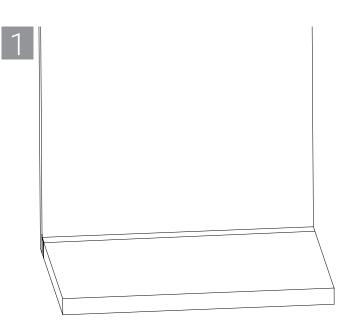
Areas to be protected must be clean and free of oil, loose dirt, rust or scale. Installation temperature shall be between 40°F (4°C) and 95°F (35°C). Consult appropriate manufacturer's drawing for system design requirements. Forming or packing materials are required as an integral part of various system designs.
