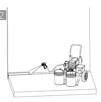
Coating may be applied by airless spray in a single pass as thick as 3/16" (4.8 mm) wet coating depth, although coating thickness requirements vary according to individual design.
