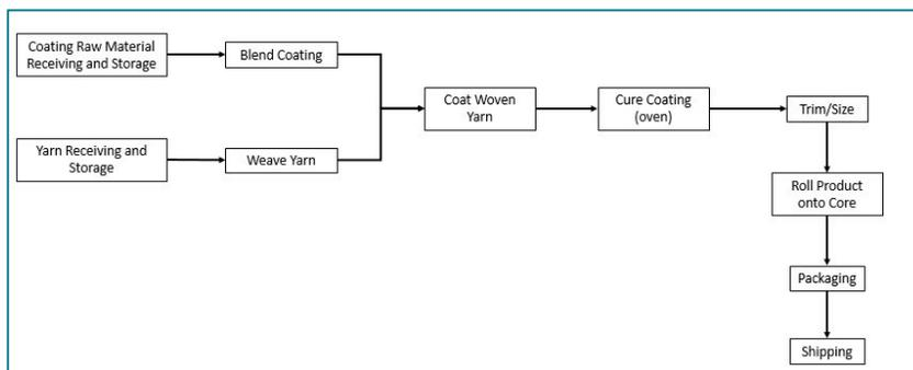
Figure 1: EIFS Mesh Process Flow
