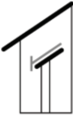
2. Kick-out flashing at lower roof terminations
