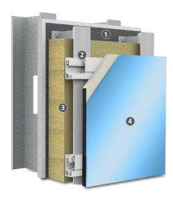
Structural Back-up Wall (by others): Steel or wood frame with glass mat gypsum sheathing in compliance with ASTM C1177, code compliant OSB or plywood sheathing, concrete or concrete masonry, existing structurally sound, uncoated brick or other
