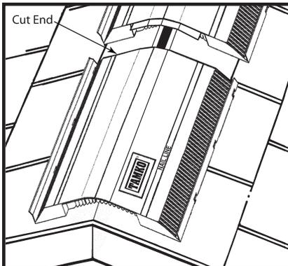
**4.** Place first cap shingle over vent so that it overhangs at least 1" over end of vent section. Install with 2-1/2" nails in nail line area as you work your way down the roof. Cut last cap shingle so that it overhangs vent 1" at other gable end.
