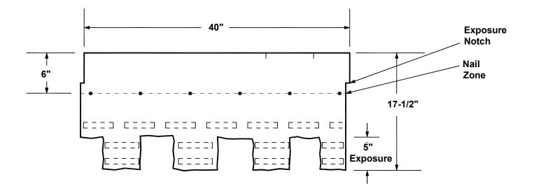
DETAIL B – 13-1/4" X 39-3/8" Overall Dimensions and Nailing Pattern
