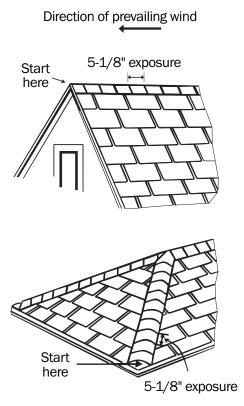
Secure each shingle as illustrated in Figure 2 with one fastener on each side, 5-5/8" back from the exposed end and 1" up the from the edge. DO NOT NAIL BELOW THIS LINE 1" UP FROM THE EDGE. The length of the fastener should be long enough to penetrate through the roofing material and 3/4" into the wood decking or completely through the decking.
