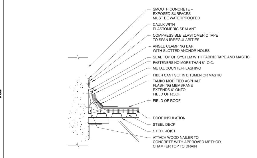
COUNTERFLASHING FOR CONCRETE WALLS OR PARAPETS
