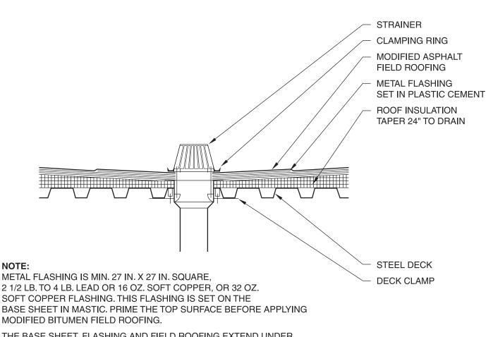
THE BASE SHEET, FLASHING AND FIELD ROOFING EXTEND UNDER THE CLAMPING RING, NO SEAMS ARE TO INTERSECT THE DRAIN. THIS DETAIL FOR USE WITH AWAPLAN PREMIUM, AWAPLAN PREMIUM FR, AWAPLAN 170, OR AWAPLAN 170 FR ROOFING SPECIFICATIONS ONLY.
