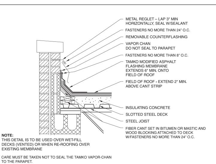
**BASE FLASHING FOR VENTED BASE SHEET**
