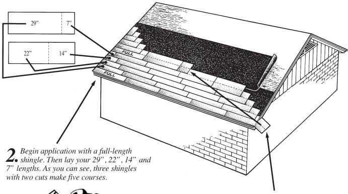
Continue working your way across the roof. When you make your final cut at the roof's edge, flip any pieces that are 8" or longer back onto the roof. These pieces can be worked in anywhere without creating zippers or color variations.
