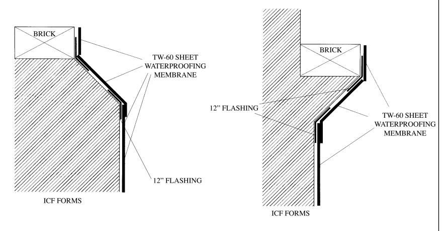
AT THIS AREA USE FLASHING STRIP DO NOT EXTEND TW-60 THRU PLANE CHANGES
