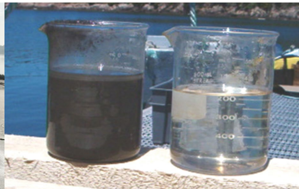
Aquaculture benthic deposit water before and after GEOTUBE ® treatment.
