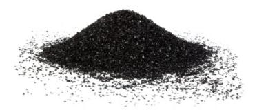
In the case of colored geomembranes such as reflective geomembranes, following the pyrolysis, the residual material weighed in the dish is a combination of carbon black and titanium dioxide. As for conductive-backed geomembranes, the weighed residual material is carbon black but in ranges that can sometimes be outside of the ranges of the GRI-GM 13 and GRI-GM 17 specifications.
