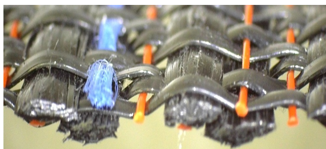
Figure 5: Cross sectional diagram and photo of MIRAFI RS380i and RS580i, illustrating wicking yarn and orange monofilament yarn placement
