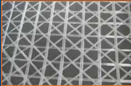
Mirafi® MPG4 Paving grid of multi-axial fiberglass attached to a light-weight paving fabric that forms a waterproof interlayer with high levels of multi-directional 360° tensile reinforcement that provides greater delay of reflective cracks.
