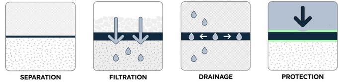
MIRAFI® S1000 is a needlepunched nonwoven pervious geotextile composed of at least 95% by weight of long-chain polypropylene fibers, which are formed into a stable network such that the fibers retain their relative position. MIRAFI S1000 is inert to biological degradation and resists naturally encountered chemicals, alkalis, and acids.
