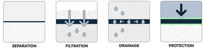
MIRAFI® S1600 is a needlepunched nonwoven geotextile composed of polypropylene fibers, which are formed into a stable network such that the fibers retain their relative position. MIRAFI S1600 is inert to biological degradation and resists naturally encountered chemicals, alkalis, and acids.
