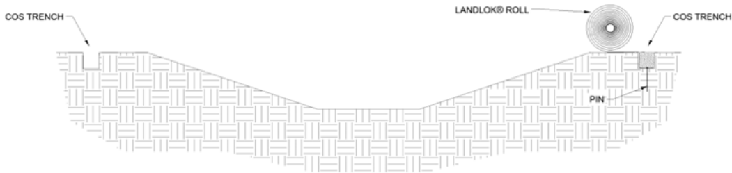
Figure 11: Perpendicular Placement of PROPEX Landlok TRM across Channel
