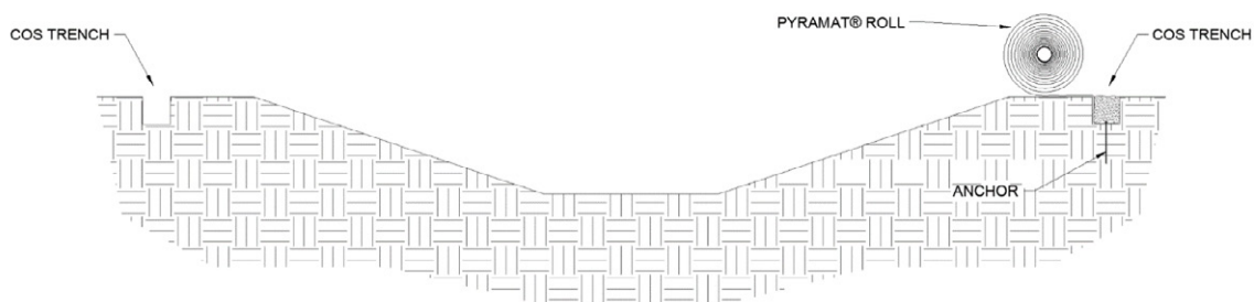
Figure 9: Top of Bank (COS) trench placement
