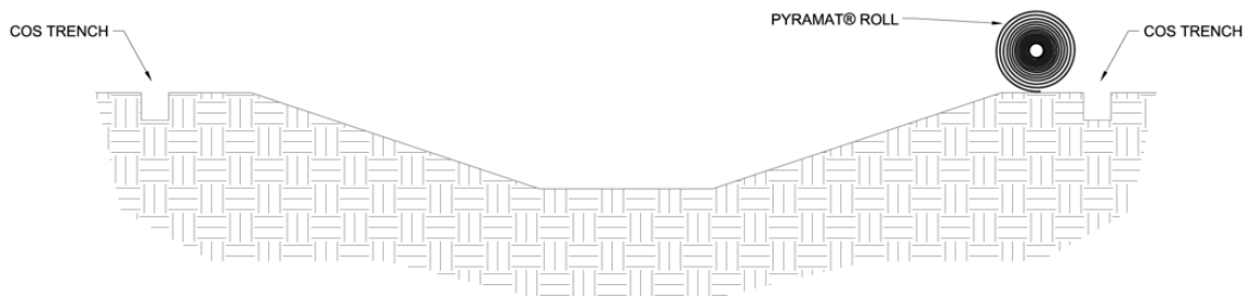
Figure 8: Top of Bank (COS) trench alignment
