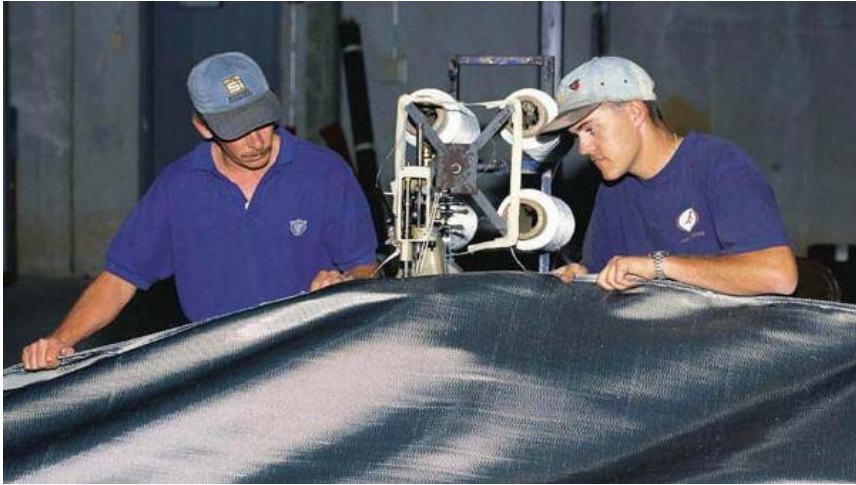
Figure 3. Factory sewing with double-needle machine
