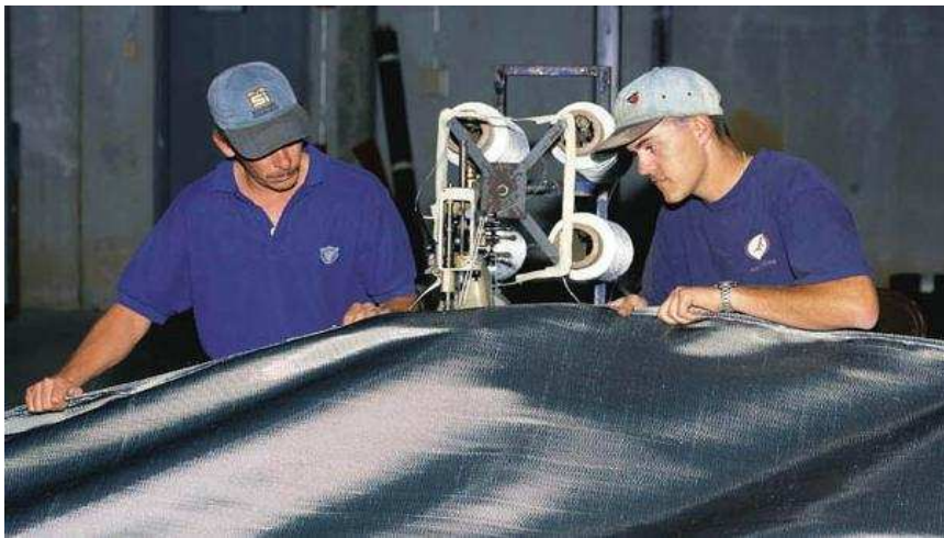
Figure 4. Factory Sewing with double-needle machine
