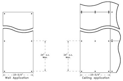
For wall applications of 31-3/4" Tectum panels, space the screws at 24" o.c. along the length and at the top and bottom of the panel perpendicular to the panel direction. Three screws per panel width are required. Locate the screws 1" to 2" from each panel edge and centered. Use the same screw pattern for ceiling applications.
