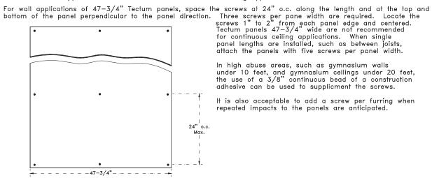
In high abuse areas, such as gymnasium walls under 10 feet, and gymnasium ceilings under 20 feet, the use of a 3/8" continuous bead of a construction adhesive can be used to supplicment the screws.
