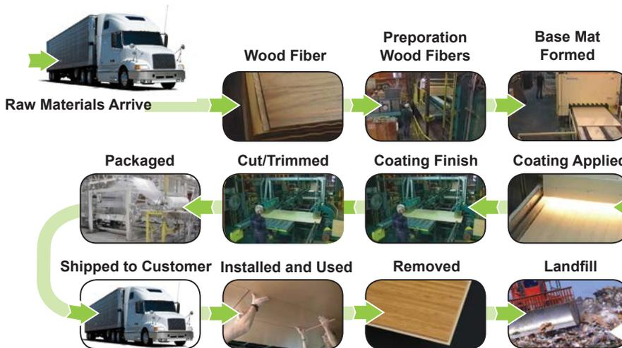
Aspen wood fibers are shipped to the plant in bales (similar to hay bales) and “combed” and separated. The fibers are then coated with a binder solution to form the base mat. The conveyor assists in forming, and creates the outer edges of the base mat. A tenor board then flattens the top of the mat, and once a base is formed, a final coat of binder is applied.
