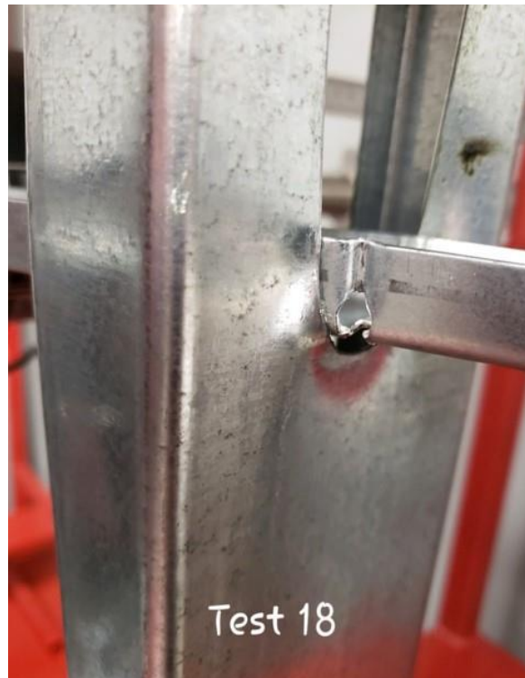
Figure 6-2: Photograph of Failure Mode for Rotational Loading
