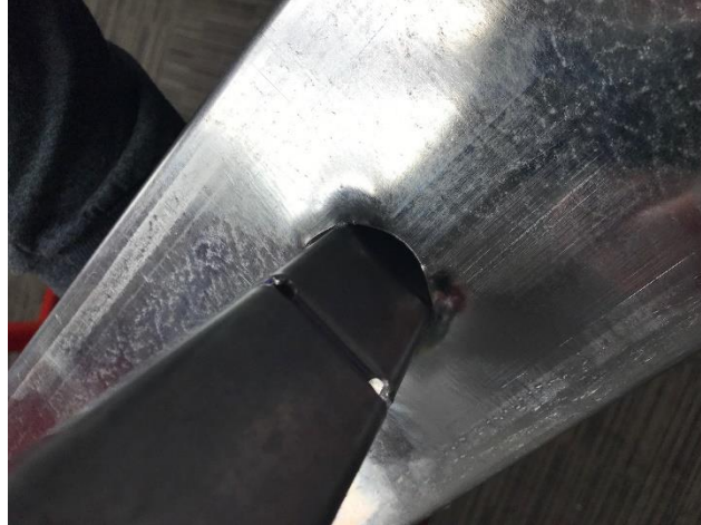
Figure 6-1: Photograph of Failure Mode for Lateral Loading
