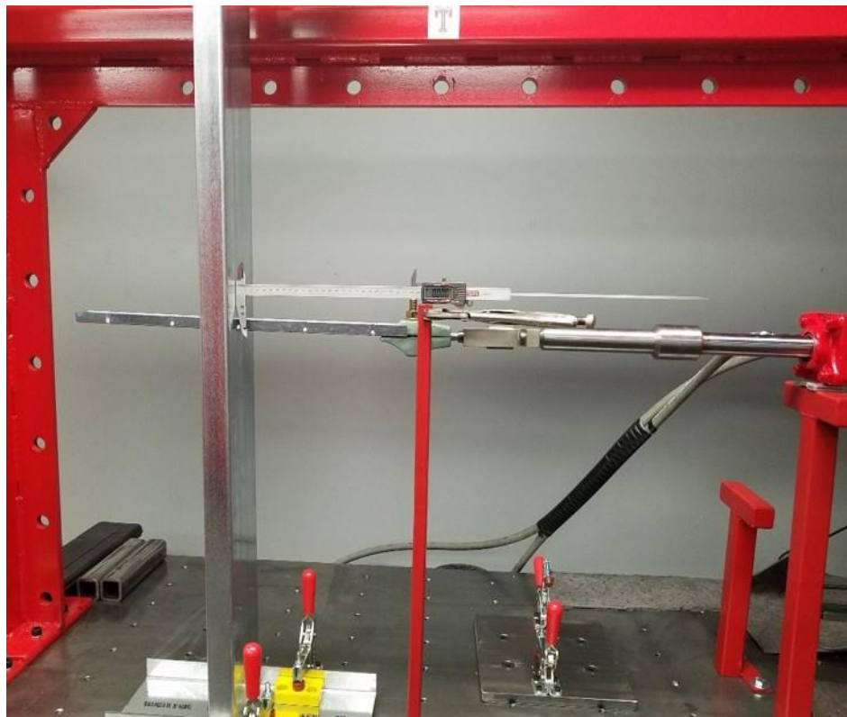
Figure 5-1: Photograph of the Lateral Loading Test Set-Up
