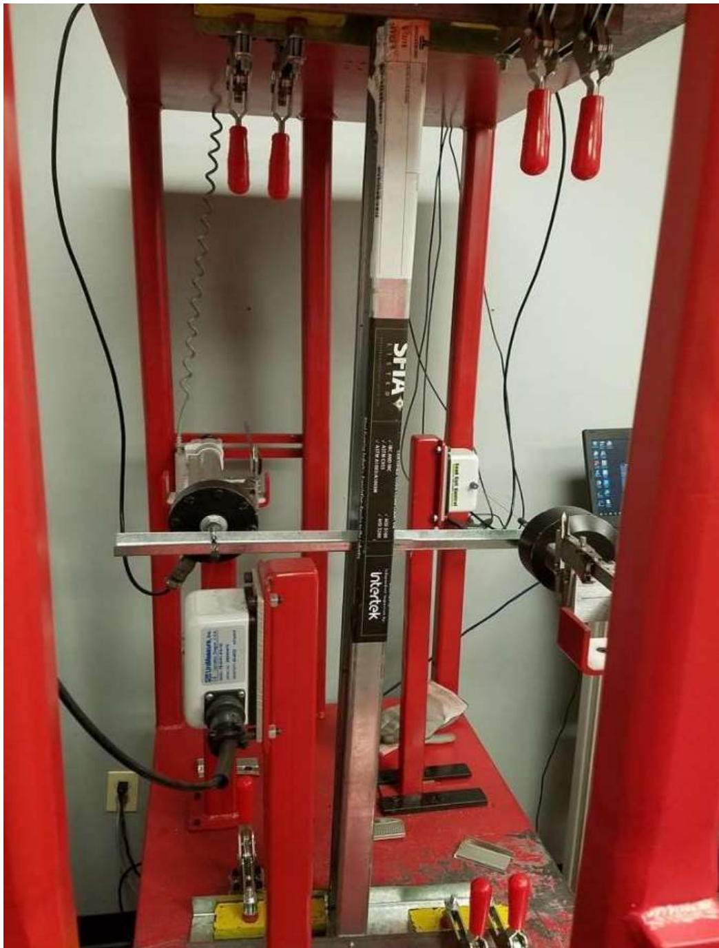
Figure 4-2: Photograph of the Rotational Loading Test Set-Up
