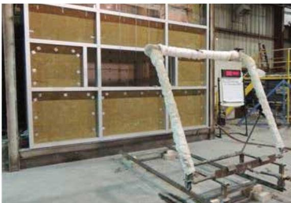
*ASTM E2307 intermediate scale, multi-story, test furnace and the test wall
