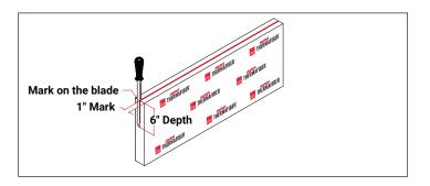
4. Continue cutting down the length of the insulation at the center of the top edge and at a depth of 6" until the end is reached.
