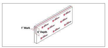
5. Next, measure down 6" and then make a 1" horizontal cut into the board down the entire face of the insulation panel.
