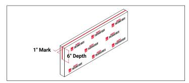
3. Insert knife into the board at the 1" mark and push the knife into the edge of the board until the top edge of the insulation meets the mark on the knife. This should make the 6" bisected cut.
