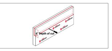
6. Once cutting is complete, the insulation board should look like the illustration below.
