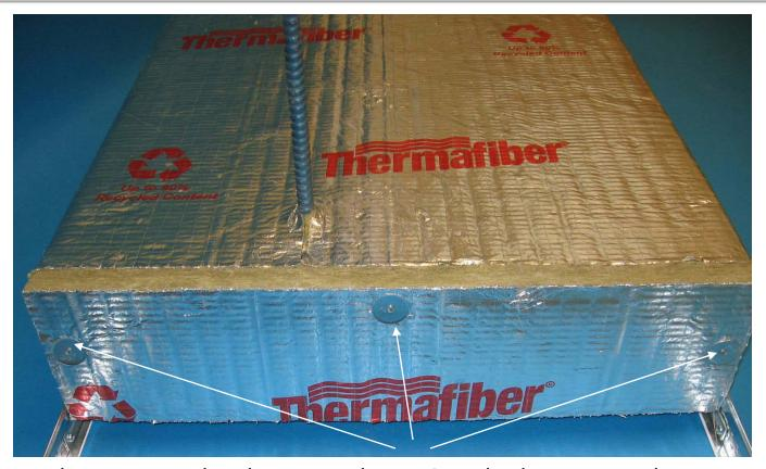
End caps secured with 4.5" steel pins. Standard cover sizes have 3 pins per cap, large covers include additional pins. Contractors report installation in about <u>6 minutes</u>.
