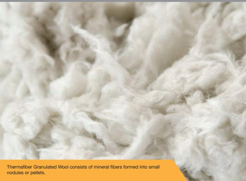
Thermafiber Granulated Wool consists of mineral fibers formed into small nodules or pellets.
