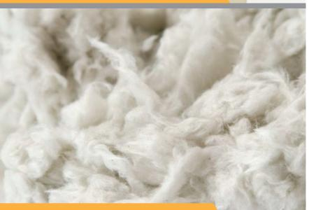
Thermafiber Granulated Wool consists of mineral fibers formed into small nodules or pellets.
