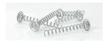
Thermafiber® Spiral Anchors are designed for easy attachment of the Thermafiber® FireSpan® mullion covers to the FireSpan® spandrel insulation panel. Spiral Anchors can be used in conjunction with the Thermafiber® Impasse® Insulation Hanger System for quick and easy installation. Spiral Anchors are also a versatile component that can be used to mechanically fasten insulation to insulation in other applications.
