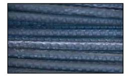
Made from low carbon steel that meets ASTM A1064 / A1064M standards. Plain or deformed wire.
