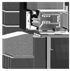
Sill condition showing Extruded Silicone Double Ribbed ETA Connection attached at the sill and corners with Spectrem 1 Silicone Sealant. The Ribbed Silicone Sheet is folded into the glazing pocket and at the corners it is folded and mechanically fastened under the pressure plate.
