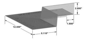
d. Extruded Aluminum Adaptor: Alodine finished extruded aluminum race for engaging darts of Proglaze ETA components. The Extruded Aluminum Adaptor is supplied in 5' lengths with pre-applied Tremco 440 tape and predrilled holes every 6" O.C.
