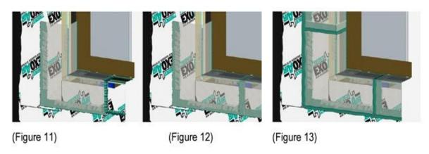
5.12 Silicone sealant is applied at the Proglaze ETA Silicone Rubber Extrusion's cut end for bonding within the 1" (2.5 cm) overlap with the Proglaze ETA Silicone Molded Corner. The Proglaze ETA Silicone Molded Corner is bedded into the silicone sealant at dart, leading edges and within overlap. See figure 13.
