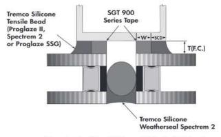
T = Sealant/Tape Thickness 1/4" min. (6.35mm) SCD= Surface Contact Depth 1/4" min. (6.35mm) W = Width of Tape (Adhesive side)
