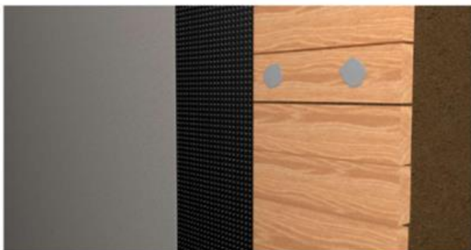
Ref 3 – Paraseal installed over TremDrain
