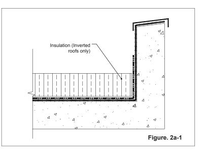
b. Cut insulation to fit neatly at projections and terminations with less than 1" (25 mm) tolerance.
