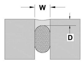
EXPANSION JOINTS - The minimum width and depth of any sealant application should be 1/4" x 1/4" (6 mm x 6 mm). The depth (D) of sealant may be equal to the width (W) of joints that are less than 1/2" wide.
