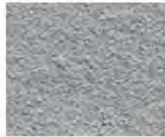
CSP 1 (Acid Etched)
