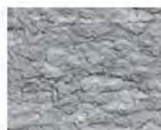
CSP 6 (Medium Scarification)
