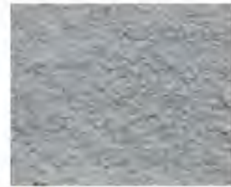
CSP 3 (Light Shot blasting)
