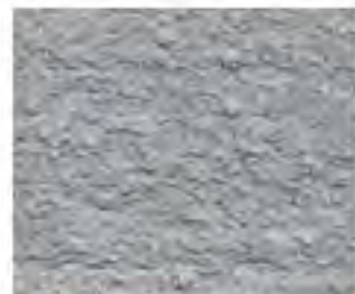
CSP 4 (Light Scarification)
