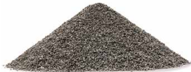
7.7 lbs granule loss per roll Acceptable per ASTM D4977
