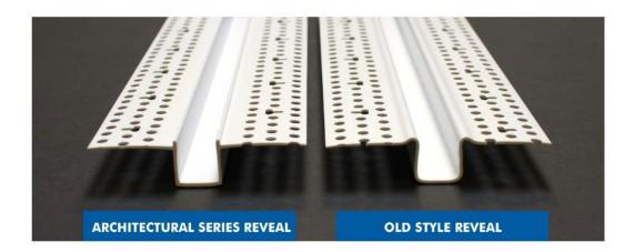
Trim-Tex has introduced the <u>Architectural Series Reveal</u>, featuring a sharp mud bump for a clean finished edge compared to the rounded edge of the original design. When installing Trim-Tex Reveals it is important to make sure that the two styles are not mixed, as the profiles will not match up. Look for the Architectural Series name to be sure you have the new sharp edge design.
