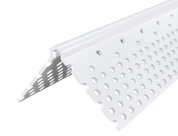
**Description:** Achieve the soft, slightly rounded edge of a standard Trim-Tex Corner Bead with a tighter 81-degree angle that conquers uneven framing, and a unique hole pattern that saves you mud and time. With Closed Angle Corner Bead's more acute angle comes an increased rigidity, giving many installers the feeling of using a metal corner bead – but with all the durability of Trim-Tex's top-quality vinyl materials.
