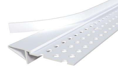
**Description:** Trim-Tex Deflection Bead is designed to prevent inside corner cracking when installed against a ceiling or concrete deck that may be subject to up to  $\frac{7}{16}$ " movement.
