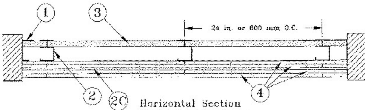
1. **Floor, Side and Ceiling Runners** — "J" - shaped runner, min 2-1/2 in. deep (min 4 in. deep when System C is used), with unequal legs of 1 in. and 2 in., fabricated from min 24 MSG (min 20 MSG when Item 4A, 4B, 4C, 4D or 7 are used) galv steel.
